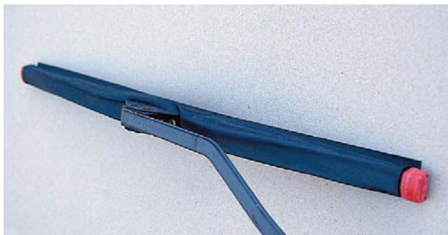
Winter wiper blades have rubber covers over their mechanism.
