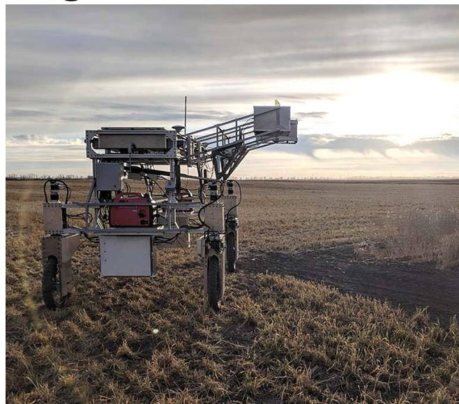
The Phenotype Acquisition and Measurement Machine (PAMM), a robotic imaging platform developed for field crop phenotyping, collects data on wheat, lentils and canola phenotypes. Photo by Tyrone Keep, USask.
