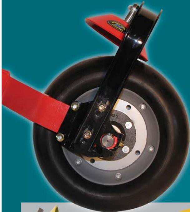
**Devloo Roto Mud Scrapers** are designed to improve efficiency and yield. Our product is laser cut from #80 steel with a 6203 NTN motor grade bearing, and powder coated for a durable finish.
