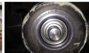
No trace of sulphur dust on the bearing after the test
