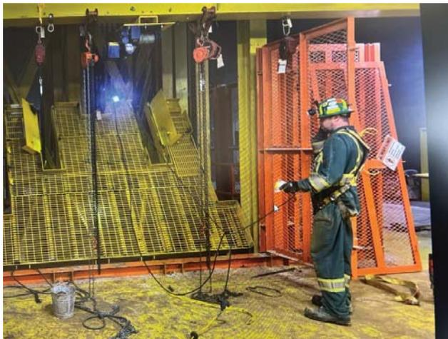
Above and below: The drawbridge that is electrically lowered by a tugger/winch system. This covers the shaft area opening while allowing access to the Blair ropes.
