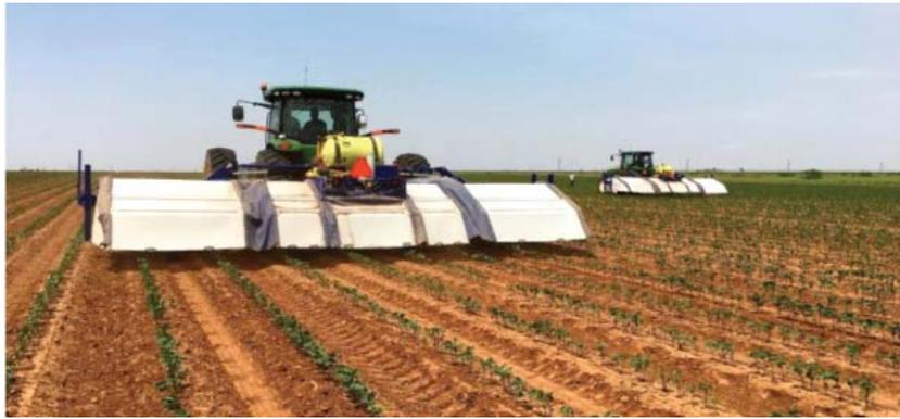
John Deere has acquired Blue River Technology, maker of 'smart' machines like the See & Spray, which uses artificial intelligence to identify weeds and robotic sprayers to dose them with herbicide. (Blue River Technology)
