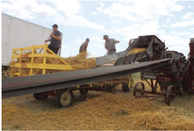
Volunteers pitching grain sheaves into the museum's antique threshing machine. The power of the machines comes from a canvass pulley belt turned by the fly wheel on a nearby tractor.
