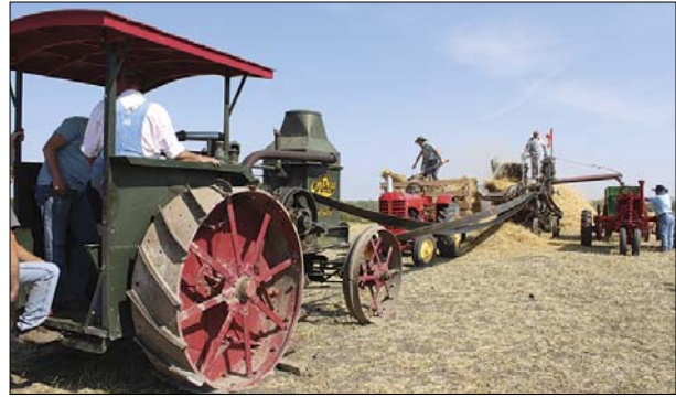
Darwin Fedorowich operating his Rumley kerosene tractor that turns the long pulley belt that turns the gears in the threshing machine at the old time harvest held at Ken and Anne Wilson's farm near Wawota.
